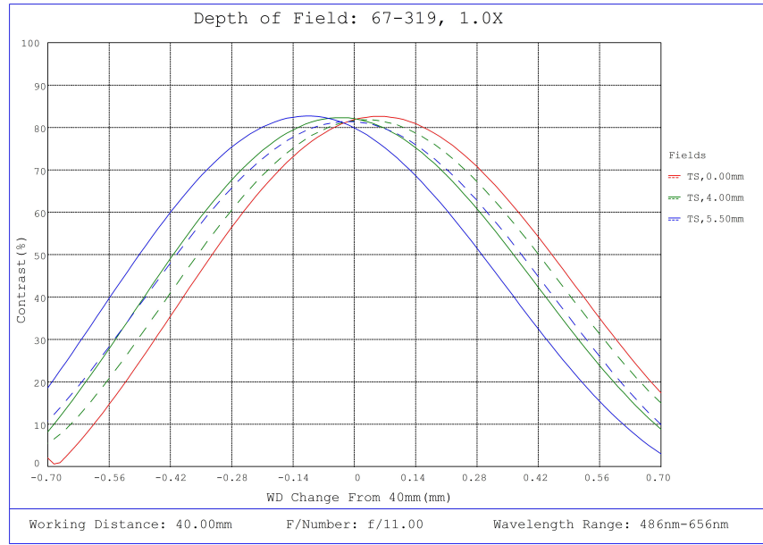
#67-319, 1X, 40mm WD, In-Line CompactTL™ Telecentric Lens, Depth of Field Plot, 40mm Working Distance, f11
