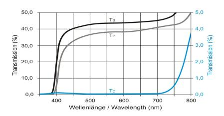
The XP42 is a high quality, neutral grey polarizer sheet of the newest generation. Through its high transmission and polarization of 400-700nm (i.e. within the visible region absorption spectrum) the polarizers can be used for many different types of applications.
