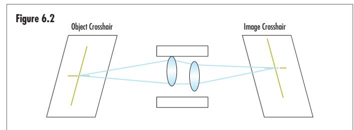
**Figure 6.2:** Perturbed system where lenses are decentered within the barrel and the optical pointing stability changes. Object crosshair is mapped to a different place on the image.
