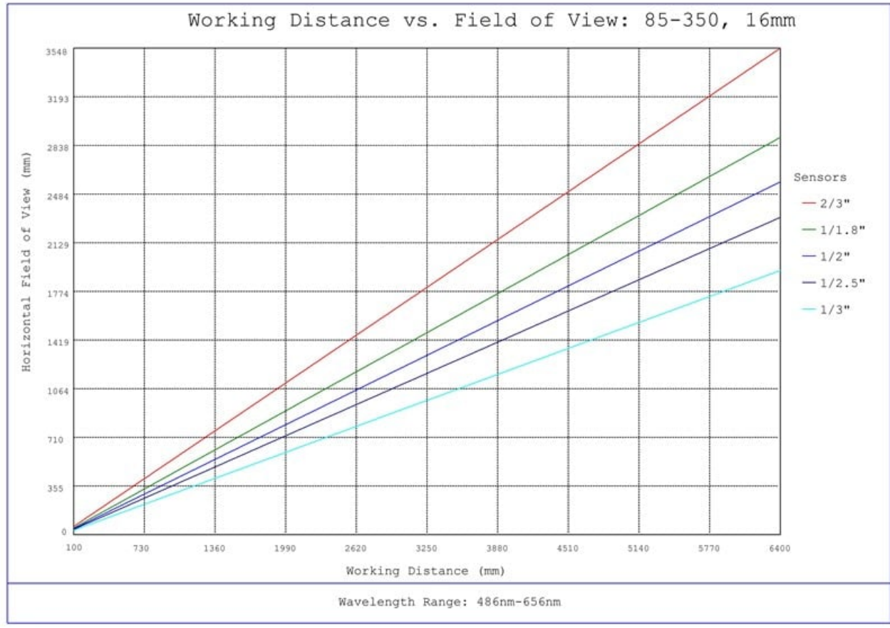
#85-350, 16mm, f/2.8 Ci Series Fixed Focal Length Lens, Working Distance versus Field of View Plot
