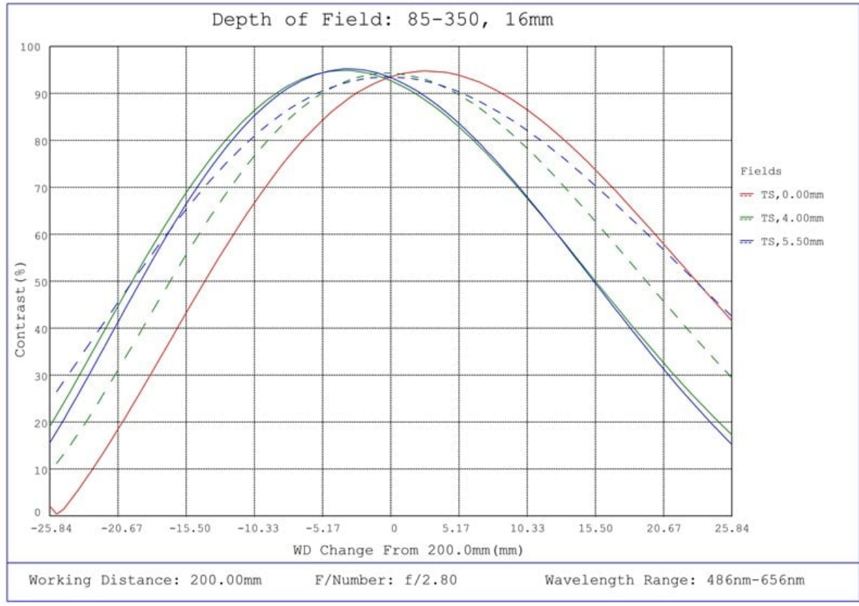
#85-350, 16mm, f/2.8 Ci Series Fixed Focal Length Lens, Depth of Field Plot, 200mm Working Distance, f2.8
